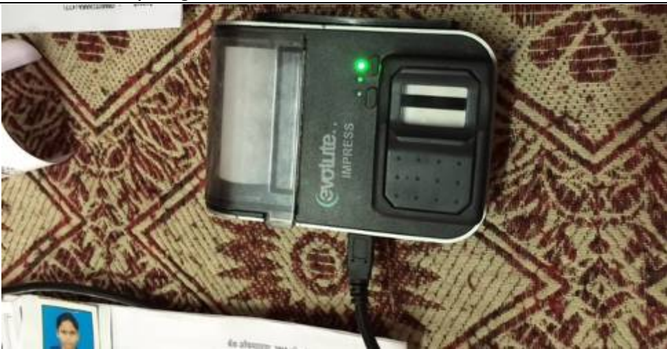
Figure 20: MicroATM with fingerprint reader which helps authenticate transactions and enables account opening in a minute for Aadhaar holders
